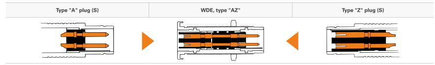
The "ZA" version of the WDE accepts a type "Z" plug at the flange side and accepts a type "A" plug at the threaded end.
